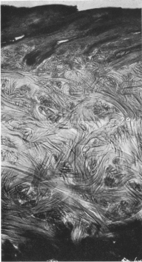
Figure 17 Strong upper leather 2 mm thick tearing at 22 kg load.
