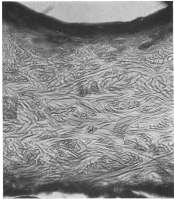
Figure 27 Upper leather after compression \times 55 .
