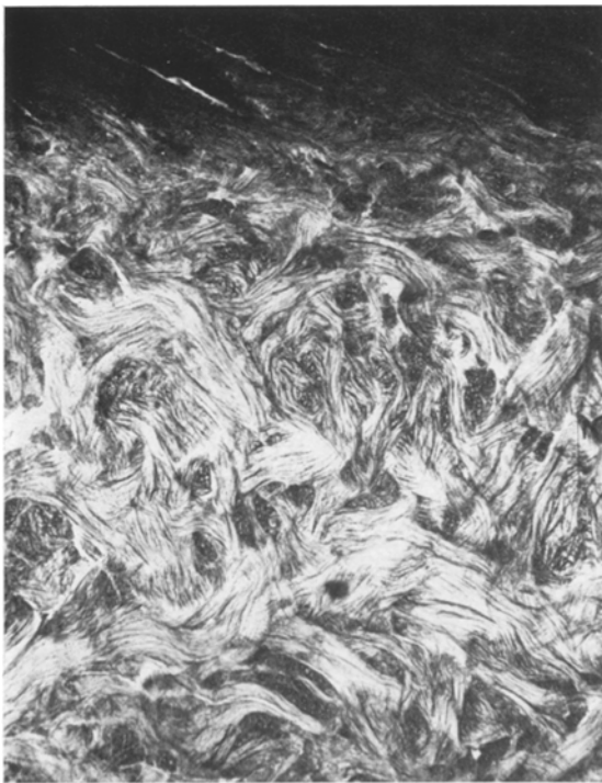
Figure 5 Vertical section through leather from cattle skin at the back of the animal, \times 20 .
