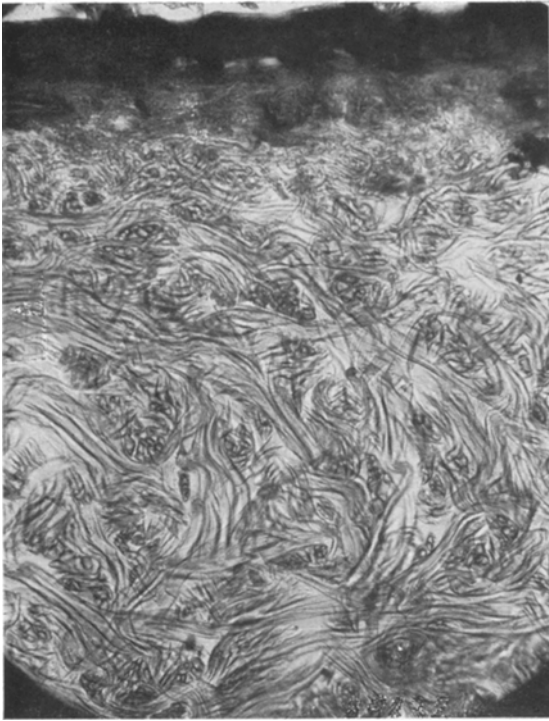
Figure 26 Upper leather before compression, \times 55 .
