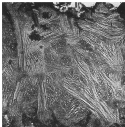
Figure 22 Weak middle split – high angle of weave insufficient interweaving, × ~ 50.
