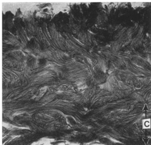
Figures 20-23 Shoe suedes made from flesh splits. Figure 20 Strong flesh split – flesh layers (C) retained, × ~ 50.
